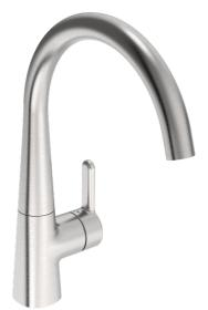
Kitchen faucet with smart dishwasher valve and high swivel spout. Spout's swing angle is factory preset at 120° (can be limited to 0° or 60°). Dishwasher valve closes automatically after 4 or 12 hours (one push opens the valve for 4 hours, pushing for 5 seconds opens the valve for 12 hours). Battery operated, 3 V. There are also in-built limitation options for water temperature and maximum flowrate. F = with flexible pipes
