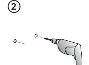
Using a 6mm drill bit, drill holes on the marked positions.
