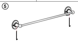
Insert the Towel Rail body into the base. Fix it with the allen key supplied.
