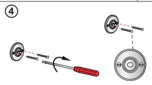
Screw in the stainless steel screws to secure the base to the wall.
