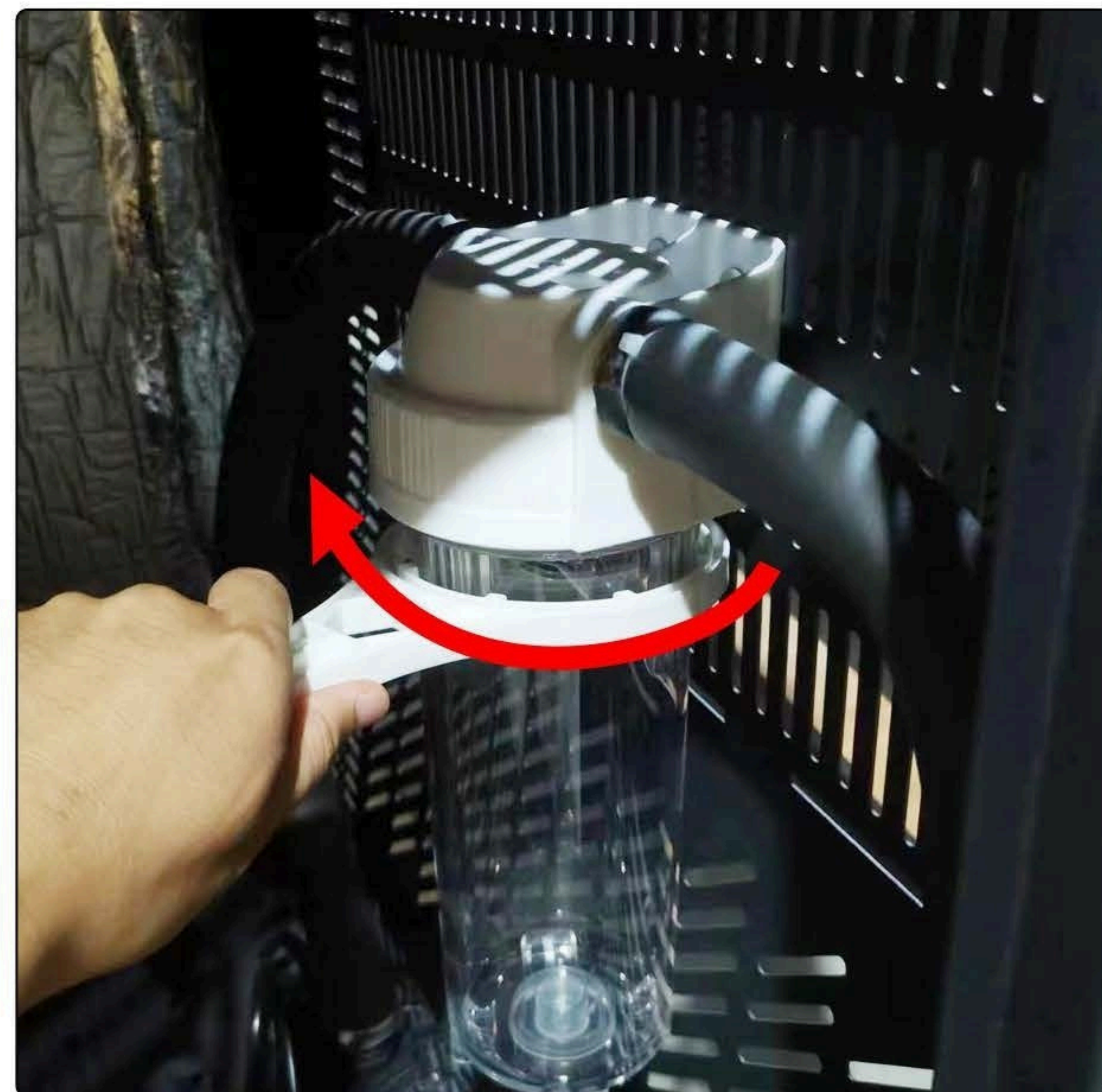
Remove the filter using a special wrench
