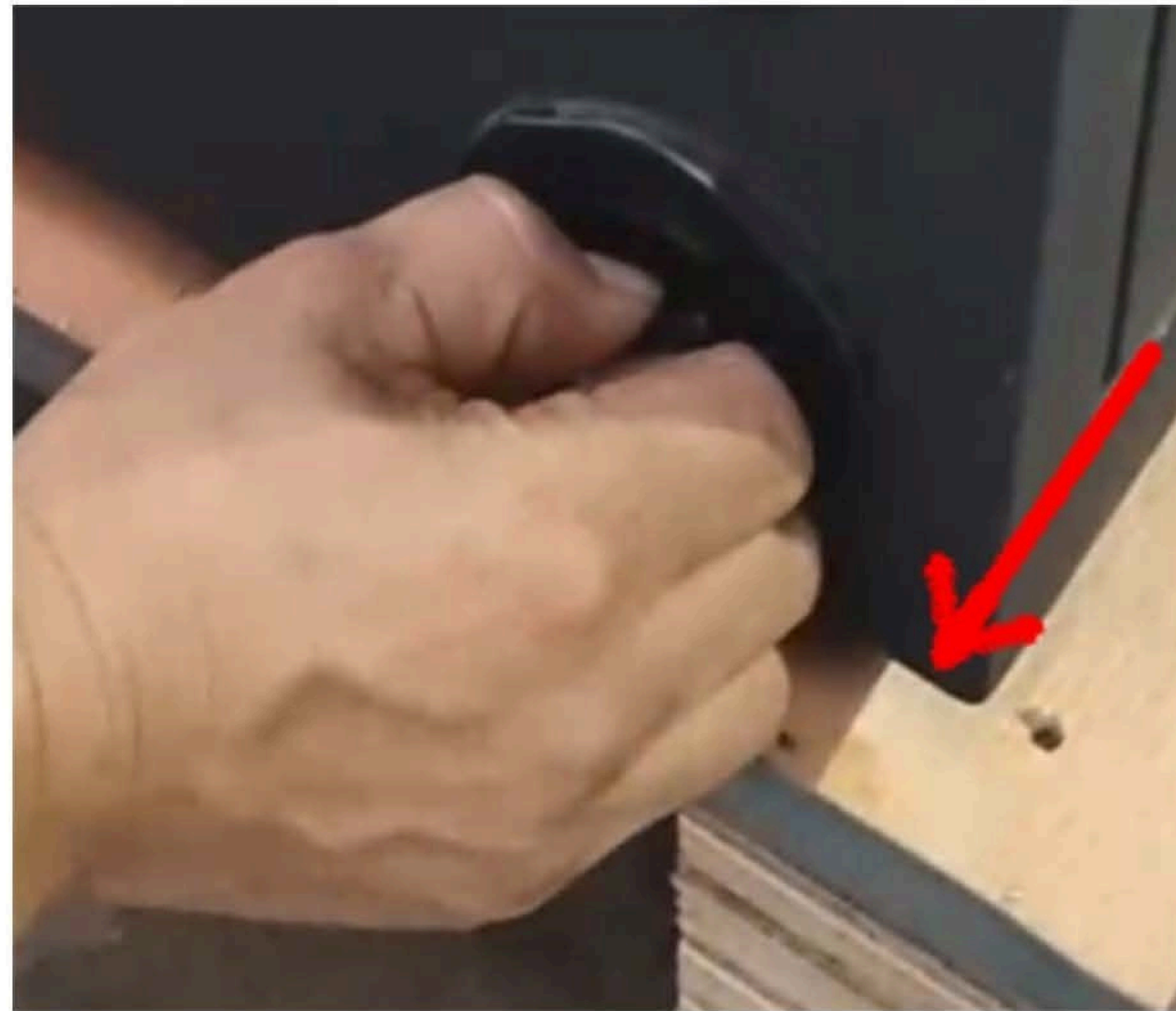
Pull out the water outlet
